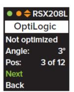
Upon completion of optimization, settings for all RSX line array modules in the array are adjusted for optimum performance across the specified coverage area. Equalization adjustments are made to compensate for low frequency coupling depending upon the number of modules in the array. Additional EQ is applied to compensate for high frequency energy loss between each module and its defined coverage area.
